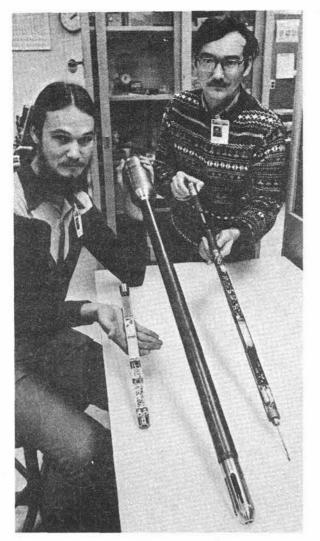
FOR GEOTHERMAL WELLS—New logging instrument which measures downhole temperatures up to 300°C is displayed by Kyle White and Dave Palmer (both 2151). Two versions of the electronics have been tested—hybrid thick film technology (which Kyle holds) and a system using printed circuit boards.
